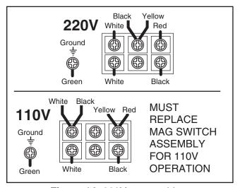
Figure 14. 220V motor wiring.
